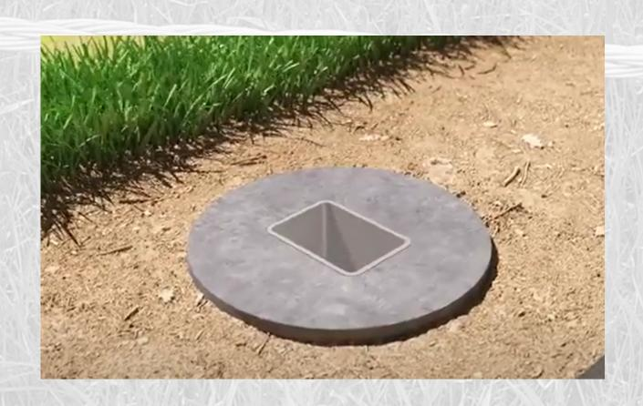
3) Insert the socket at an angle so that when TP1-4 is placed in the socket, the post is 1-1/4" per 12" out of plumb. Socket and post should lean towards the CRP.
